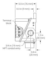
The nVent RAYCHEM AMC-1A ambient-sensing thermostat is designed to control heat-tracing systems used for freeze protection in nonhazardous locations. The thermostat responds to ambient temperature changes and has an adjustable set point. The AMC-1A can be used to control a single heat-tracing circuit or as a pilot control of a contactor switching multiple heat-tracing circuits.
