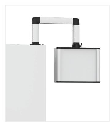
The mild steel operator interface control enclosure, OICE, has a pre-machined hole pattern to allow for the fixation to a swing arm, plus a removable front plate at an IP 55 protection degree. Components can be easily fitted thanks to the removable front plate, but will also be easily accessible through a rear door. Side handles on the enclosure allow for easy movement of the enclosure into the working position.
