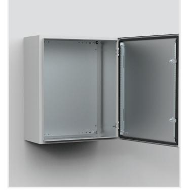
The galvanised steel single door wall mounted enclosure range, MASE, is designed to meet EMC requirements. An excellent Faraday effect is created, since electrical conductivity between the enclosure body an door is guaranteed. The risk for component failure, and with that unnecessary downtime, is eliminated as electromagnetic interference is avoided and water and dust are prevented from entering the enclosure. This enclosure range is well suited for applications where EMC is required.
