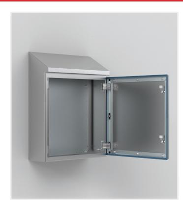
The nVent HOFFMAN Hygienic Design HDW range is designed and constructed with special materials for high sanitary operations and ease of thorough cleaning. The gapless design, the self-drainable high-polished surfaces, together with a high protection degree help reduce non operative hours, such as cleaning and maintenance, which leads to increased productivity.
