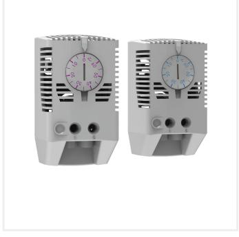
This adjustable temperature thermostat, ETR, for any enclosure, with either a normally open (NO) or normally closed (NC) contact, is used to control installed devices. Such devices could be a filter fan or a fan heater, that should turn on or off at the required temperature level, set by the user. The result is reduced operational cost.
