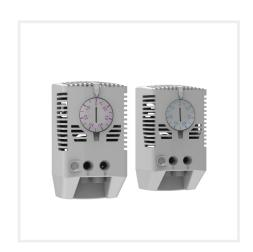
**Description:** Thermostat with NC/NO contacts to manage temperature in panels. ETR202 with a normally closed contact for regulating heaters. ETR201 with a normally open contact for regulating cooling devices or signal devices. Sensor element thermostatic bimetal. Mounting clip for 35 mm DIN rail (EN 60715).
