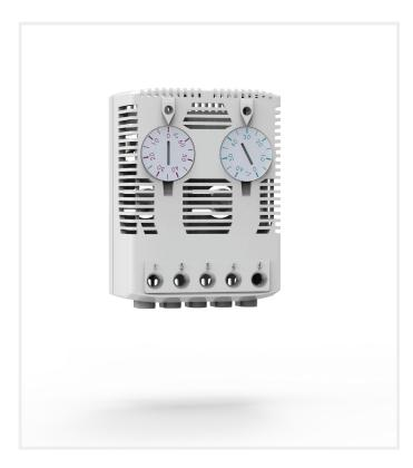
This adjustable thermostat and hygrostat, ETF300, with either a normally open (NO) or normally closed (NC) contact, manages both relative humidity and temperature. It is used to control installed devices, such as a fan heater, to turn on or off at the required humidity and temperature levels, that are set by the user. The result is elimination of water condensation at a reduced operational cost.
