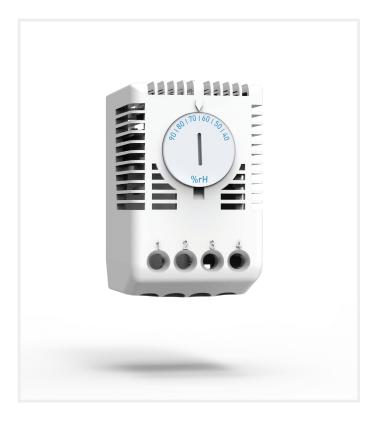
This relative humidity hygrostat is available as pre-set, ETF200, or adjustable, ETF2000. It activates a device, such as a heater, within the enclosure, either at the pre-set level, 65%, when the relative humidity has been exceeded, or at a level set by the user, which could be between 40-90% humidity.
