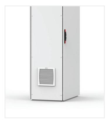
This outdoor vertical filter fan, EFP, with a polycarbonate cover and with a IP 55 protection degree, is easy to install thanks to its click-in feature. Unnecessary downtime is avoided, since water and dust are prevented from entering the enclosure through the filter, and the reliable fan motor will ensure constant ventilation. This filter fan is ideal both in indoor and outdoor environments, including direct sunlight thanks to its resistance to UV radiation.
