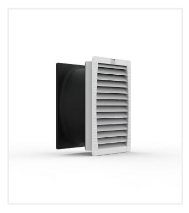
This EMC vertical filter fan, EFE, with a IP 54 protection degree, is easy to install thanks to its click-in feature. Unnecessary downtime is avoided, since water and dust are prevented from entering the enclosure through the filter, and the reliable fan motor will ensure constant ventilation. EMC performance is maintained on an EMC enclosure with this filter fan.
