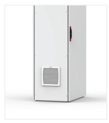
This outdoor vertical exhaust filter, EFAP, with a polycarbonate cover and with a IP 55 protection degree, is easy to install thanks to its click-in feature. Unnecessary downtime is avoided, since water and dust are prevented from entering the enclosure through the filter. This filter is ideal both in indoor and outdoor environments, including direct sunlight thanks to its resistance to UV radiation.
