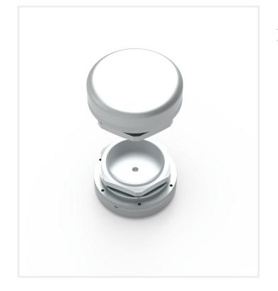
The pressure compensation plug equalises the pressure that occurs, due to temperature differences, inside the enclosure with the outside environment, while reducing the risk of dust entering the enclosure.
