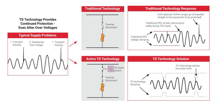
Effectively, TD Technology allows the SPD to have two clamping levels – one well above the peak of a TOV (up to twice its nominal AC voltage!), and the other much lower, to effectively and swiftly clamp lightning transients.
