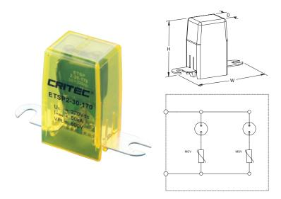
The nVent ERICO Electronic Track Signal Protector series provides transient protection from surges induced or conducted onto low-voltage signal circuits for trackside signaling equipment. The series of surge-protection devices is ideal for protecting DC-responsive track relays, train-detection systems, microprocessor-based train-control and indication circuits, train inspection systems, communications systems, highway crossing
