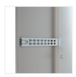
**Description:** The DIP profile system is a 40 mm wide and 25 mm high profile, which can be mounted on the enclosure depth. It can also be used in combination with CLPF and CLPK profiles. Two rows of holes patterns for cage nut fixing and self-tapping screws are provided. DIP profiles are not compatible with adjustment in depth of the mounting plate.
