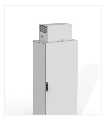
This roof cooling unit, CUH, with a IP 54 protection degree, provides cooling, either to one enclosure or to a complete assembly, depending on the cooling requirements and desired energy consumption level. It is placed on top of the enclosure and is perfect when there is not enough space on the door or side panels.
