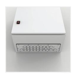
**Description:** Two-component grommet with membrane seal and cable anchorage. The installation does not require tools, it is self-adjusting to its surrounding wall thickness and click-fixed in place. Because of its compact design it only extends 5.7 mm outside the enclosure on which it is mounted. The "pushout" membrane is a permanent seal until it is penetrated by a cable or pipe. Suitable for holes in materials of 0.7 to 3 mm thickness.
