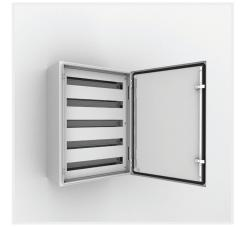
**Description:** Used for easy mounting of DIN-rail components with a maximum height of 68 mm. Distance between rows 125 mm. If required, the standard enclosure door can be replaced with a glazed door. Usable depth between front cover and external door: 35 mm. In stainless steel enclosure machining is required.
