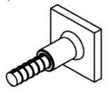
LENTON weldable half coupler provides a mechanical means of connecting rebar to structural steel plates and shapes. Coupler is manufactured from weldable grades of material. One end of the coupler is machined with a LENTON taper thread and the opposite side is prepared for welding. Weld shall be designed by a licensed design professional in accordance with American Welding Society (AWS) standards. Connection is then tightened per the manufacturer's instructions.
