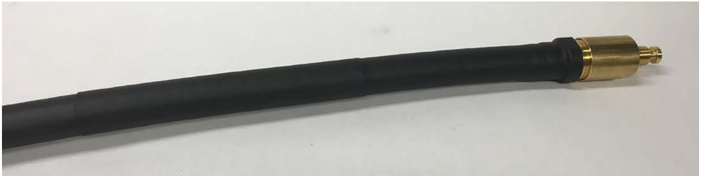
Figure 12: Heatshrink sections overlapping
