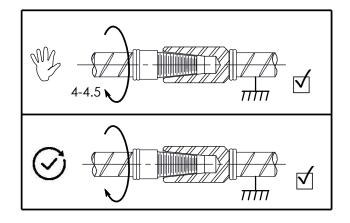
Rotate by hand to engage male and female taper threads
