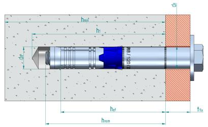
$\begin{array}{ll} d_0 \colon & \text{Nominal diameter of drill bit} \\ d_f \colon & \text{Fixture clearance hole diameter} \\ h_{\text{ef}} \colon & \text{Effective anchorage depth} \\ h_1 \colon & \text{Depth of drilled hole} \end{array}$
