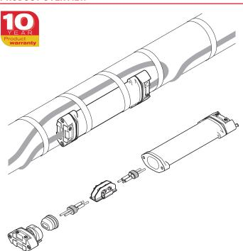
The nVent RAYCHEM S-150 is a cold applied low profile splice for in-line connection. This universal kit fits with all nVent RAYCHEM industrial heating cables, BTV, QTVR and XTVR, meaning simplified product selection and reduced inventory to stock. It can be used in applications with temperatures ranging from  $-55^{\circ}\text{C}$  to 200°C. It is approved for use in hazardous areas.
