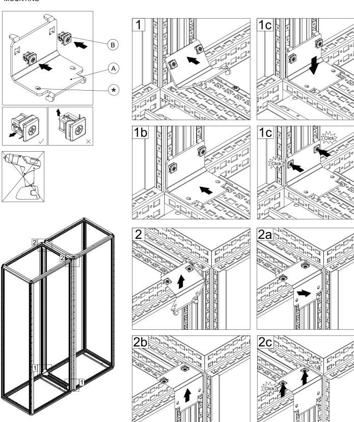
Note: It is mandatory for all four brackets to be installed at all four corners!
