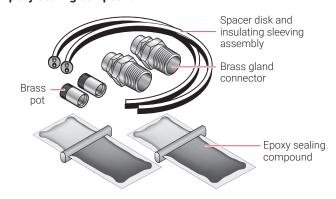
Termination type Field termination (for two cable ends)
