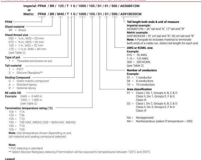
Example: Pyropak kit required for 4/14-465, four-conductor, # 14 AWG cable, for Class I, Div 1, with 12 in PVC insulated tails on both ends, and using standard epoxy sealing compound is:
