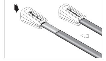
**Note:** The end seal is designed to be installed only once; it cannot be removed from the heating cable once installed. Do not use until ready for final installation.
