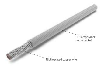
nVent RAYCHEM STS-HT Tracing Wire is a specially formulated, chemical resistant wire made specifically for high temperature STS Trace Heating applications up to 260°C. STS Systems using STS-HT Wire are ideal for heating pipelines transporting materials such as sulfur and asphalt.
