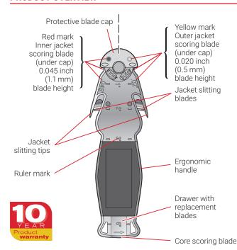
The nVent RAYCHEM Stripping-Tool-SR-Cable is designed for use with nVent RAYCHEM BTV-CR, BTV-CT, QTVR-CT, XTVR-CT, HWAT, XL-Trace, IceStop and RaySol self-regulating heat-tracing cables. The tool is designed for faster, safer and more reliable cable terminations.
