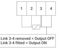
Terminals 1 to 3 allow for the connection of a three wire PT100 sensor. Terminals 3 to 4 allow the user to select the default heating status on sensor error. Without a link fitted the heating will turn OFF if a sensor error is detected. With a link fitted the heating will turn ON if a sensor error is detected (default).
