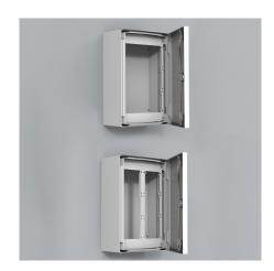
**Description:** Frame to be covered with individual cover plates UICP. For enclosures 600 and 800 mm wide it has 2 columns. Distance between UFCP and enclosure door: 39 mm; 49 mm for UCP750 and above. Reversible mounting position, to increase the distance between UFCP and enclosure door by 30 mm.
