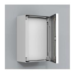
**Description:** Plain front cover plate to protect the equipment mounted in the enclosure. Distance between UFCP and enclosure door: 39 mm; 49 mm for UCP750 and above. Reversible mounting position, to increase the distance between UFCP and enclosure door by 30 mm. The cover plate can be hinged using the UHS accessory, allowing the user to gain access to components and/or cable management without having to remove the cover plate.
