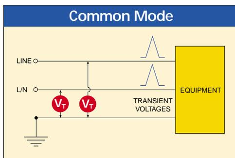
**Coupling** - Interaction between circuits, during which energy is transmitted from one circuit to the other. May be coupled galvanically (directly), magnetically or capacitively.
