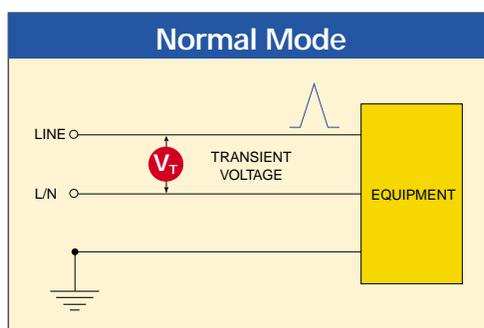
**Residual Voltage** - Another term for let-through voltage. However, some standards define residual voltage as being measured when testing is conducted with nominal or MCOV voltage applied. This is optional with let-through results.
