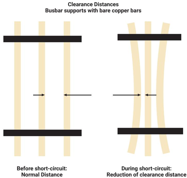
For plain bars, it requires the user to properly select the right product, using the nVent ERIFLEX Low Voltage Power Connections Software calculator, and then installing the right type and number of busbar supports to withstand a prospective fault current.
