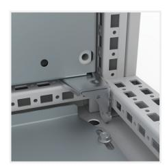
**Description:** To fix mounting plates in the enclosure, including brackets for depth adjustment in steps of 25 mm. Brackets are needed when an extra mounting plate is required or when the enclosure is ordered without mounting plate (PE).
