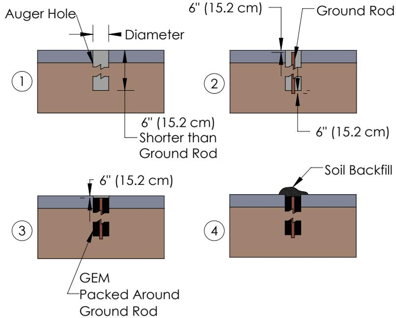
**Note 1:** Excess standing water must be removed from the trench or the augered hole before GEM installation.
