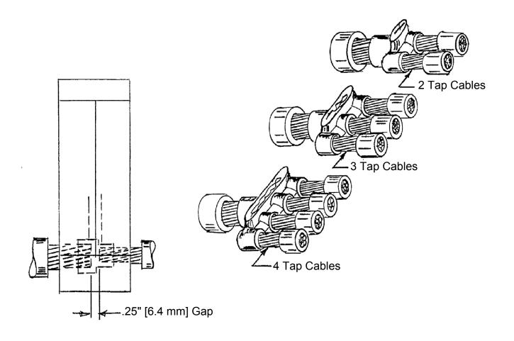
Prior to making a connection, read and follow the full instruction sheet IPRNS, IPP, and the full instruction sheet shipped with CADWELD® (IPX), and special instructions below.
