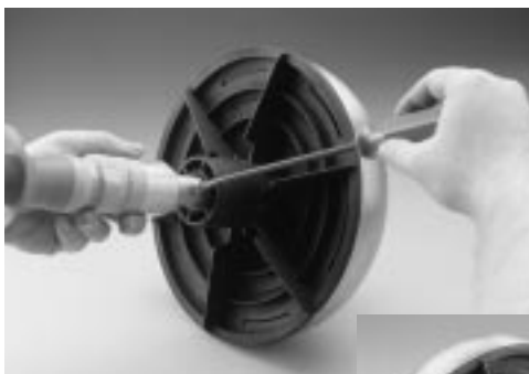
Photo 10: Once the DYNASPHERE has been fitted to the termination coupling, ensure the locking screw is tightened securely.
