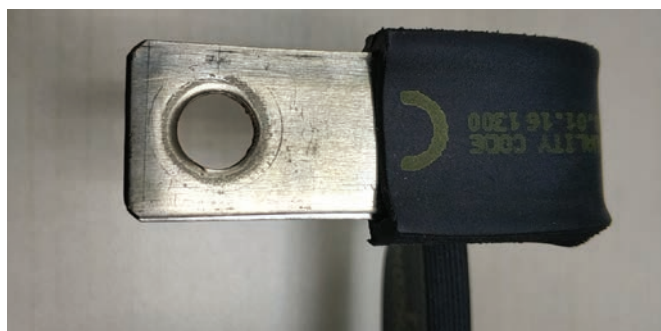
Figure 12 – Close-up shot of the nVent ERIFLEX Flexibar Advanced termination after vibration testing.
