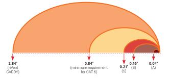
Indicate Pinch Point 0.84" Radius (minimum requirement for CAT 6) Competitor J-Hook Trace Line nVent CADDY Cat HP J-Hook Trace Line
