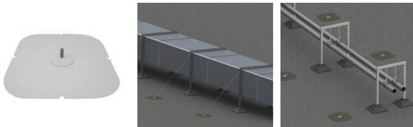
nVent CADDY Pyramid Rooftop Anchors provide an ideal method of installing rooftop anchor points for bracing applications. The installation provides a watertight membrane seal to the roof deck. Superior membrane protection compared to other evasive anchoring and ballasting techniques that can void warranties. The anchors come in TPO, PVC and EPDM single ply materials, along with modified asphalt surface.
