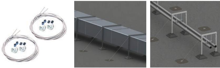
nVent CADDY Pyramid Rooftop Cable Bracing provides a safe and secure method to attach electrical and mechanical applications to rooftop anchors. Ideal alternative to rigid bracing for rooftop applications, the system includes stainless steel cable, attachment fittings, crimping sleeves and related tools.
