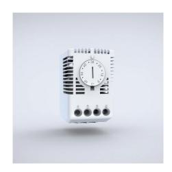
**Description:** Thermostat with changeover contact to manage any kind of device, heater or cooling. Sensor element thermostatic bimetal. Mounting clip for 35 mm DIN rail (EN 60715).
