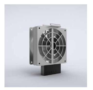
This high performance fan heater, EHV, has high heating capacity. It uses a fan to distribute the heat generated evenly throughout the enclosure, which means hot spots can be prevented. Water condensation is eliminated, also when the ambient temperature drops sharply.
