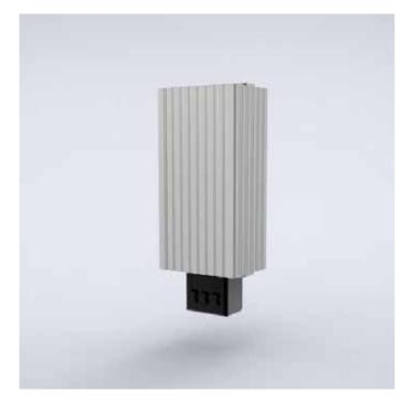
This anti-condensation heater, EHG, is available with a heating capacity range of 15-150 watts. The wide range makes it easy to find the most optimum heater also when space within the enclosure is restricted. Water condensation is eliminated, also when the ambient temperature drops sharply.
