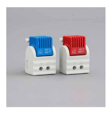
This fixed temperature thermostat, EFR, with either a normally open (NO) or normally closed (NC) contact is used to control installed devices, such as filer fans or fan heaters, to turn on or off when required. The result is a reduction of operational cost. A pre-set temperature limit prevents unauthorised personnel from tampering with the thermostat.
