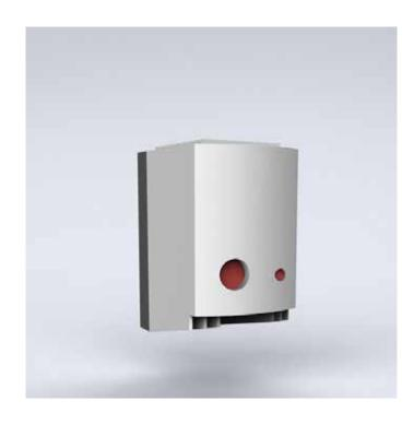
The high performance heater, ECR, with an integrated thermostat and a heating capacity of 550 watts, uses a fan to distribute the heat generated evenly throughout the enclosure, which means hot spots can be prevented. Water condensation is eliminated, also when the ambient temperature drops sharply.
