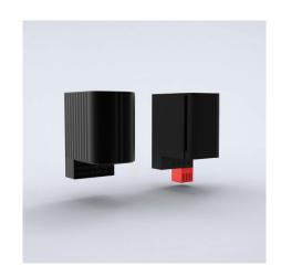
**Description:** Double insulated vertical heater to prevent condensation. Mounting clip for 35 mm DIN rail (EN60715). Touch-safe heater, the temperatures of the housing are kept under 80 °C except upper protective grille. The heater with thermostat (ECHT) includes a plug-in thermostat therefore it does not require additional wiring, starting temperature of 5 °C, and switch-off temperature of 15 °C.
