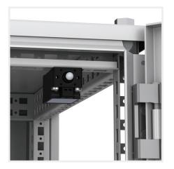
**Description:** Door switch to activate any electrical device (lighting, signalling, alarms, etc.). Can be mounted after installing the enclosure thereby keeping the door opening free. Fixed on the inside hole pattern of the enclosure's frame in floor standing enclosures. Cable entry M20.
