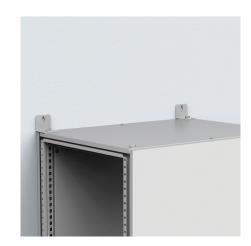
**Description:** To fix the enclosure to the wall by using M12 screws on the top of the enclosure. Prevents the enclosure from tipping over e.g. on board ships. Compatible with combinable and compact mild steel floor standing enclosure ranges.
