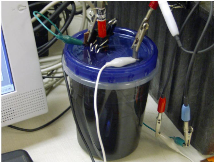
Figure 2 – Photograph of LPR Test Cell
