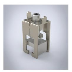
**Description:** Terminal for flat conductors with captive clamping screws, conductor can be overlapped, indication of nominal cross-section and tightening torque noted on the terminal. Contact between conductor and busbar via contact block.
