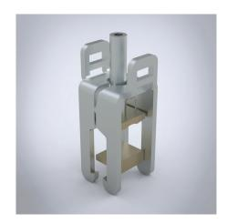
**Description:** Brace terminal, up to 300mm², for round conductors. Terminal with captive clamping screws, conductor can be overlapped. Indication of nominal cross-section and tightening torque noted on the terminal.
